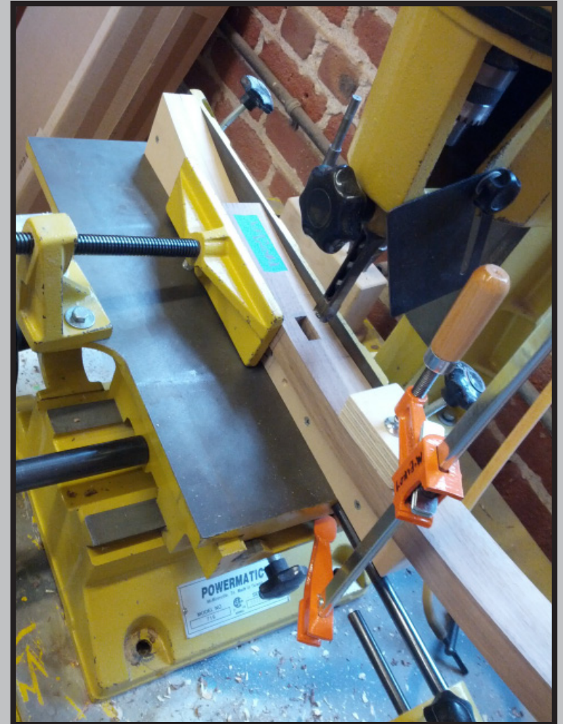
Mortising the rockers with a custom MDF jig.
