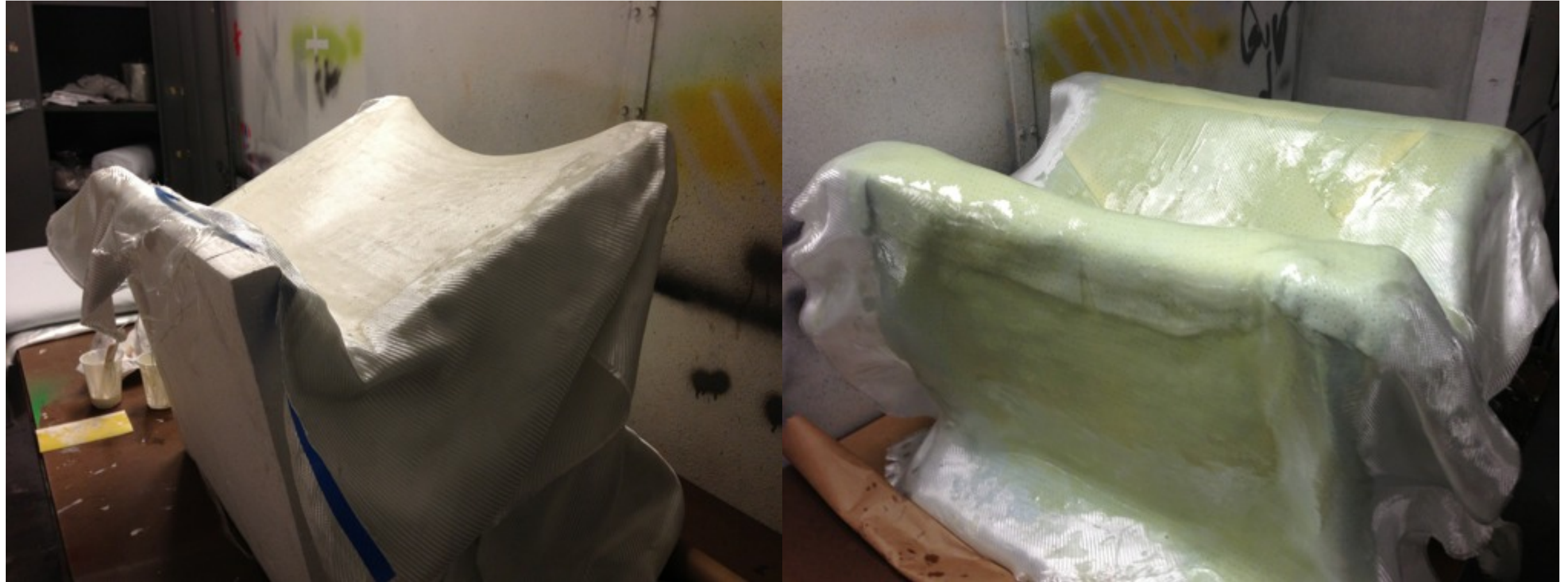
fiberglass draped over the buck at an angle
