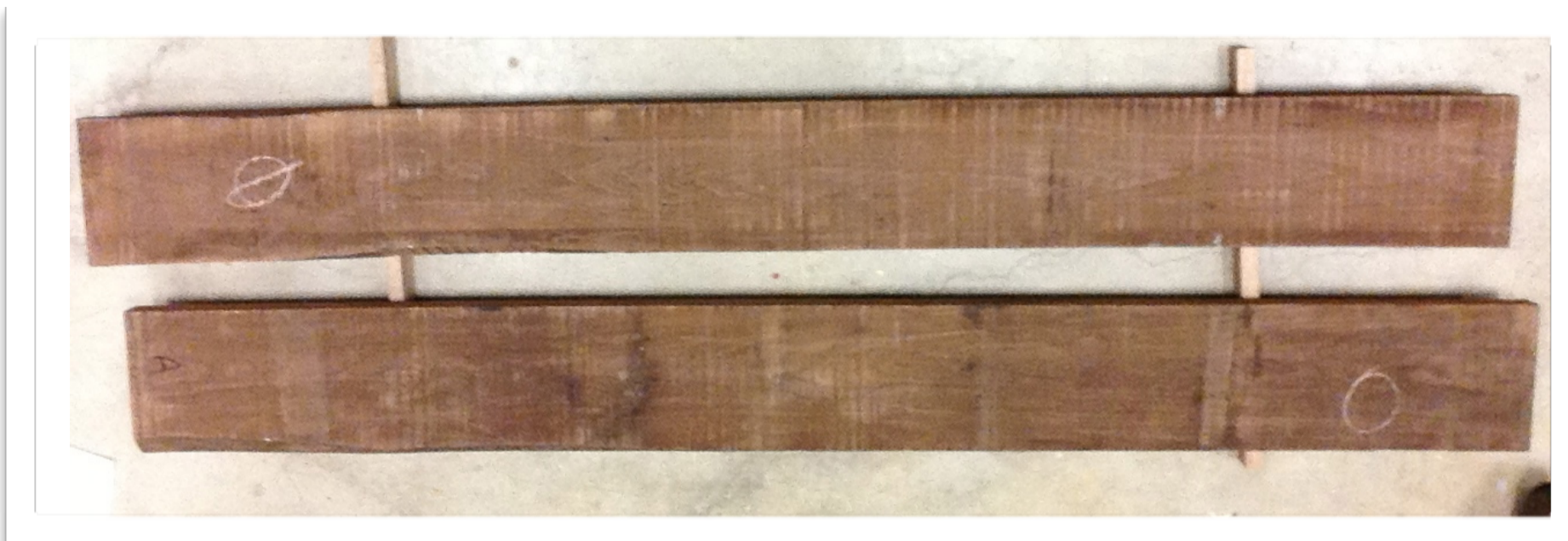
Planing for ripping the wood to size, to avoid, knots, bows and get the best possible grain running where you want in the final design
