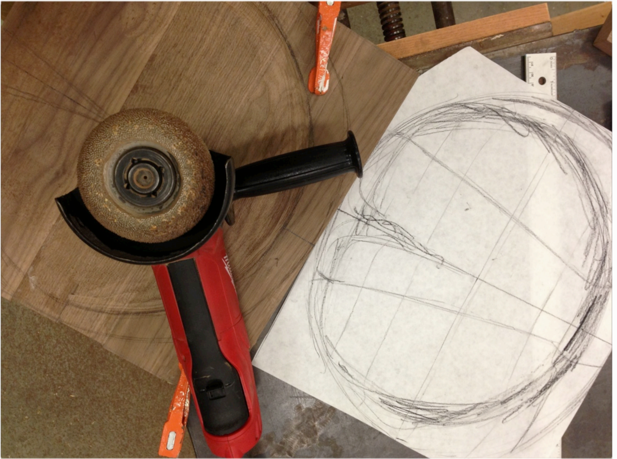
Carbide abrasive disc used to sculpt a trial piece of wood. Carving a curved line is quiet tricky. Its no work to be done when sleepy or alone late at night.
