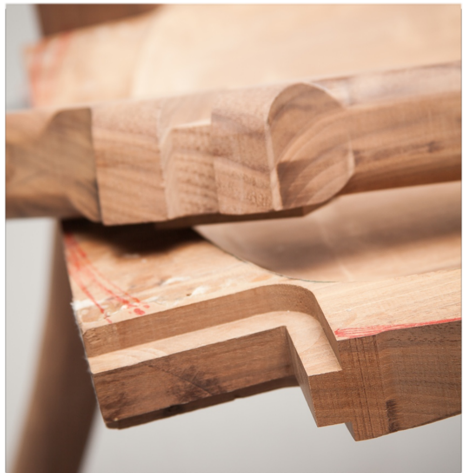
Carbide abrasive disc used to sculpt a trial piece of wood. Carving a curved line is quiet tricky. Its no work to be done when sleepy or alone late at night.
