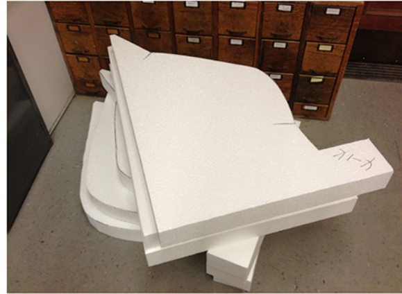
Styrofoam sheets cut to shape according to patterns. The sheets were glued together with Super77 spray adhesive.
