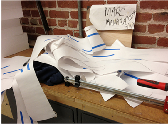
Profile patterns were cut using laser-cam on butcher paper.
