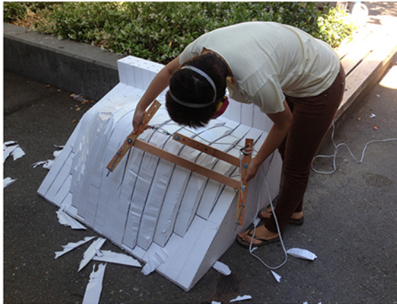
Cut styrofoam with hot wire cutter.
