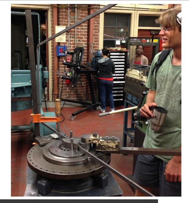
Though multiple TAs and Craig told me I was not going to be able to bend thick, rectangular steel bar on the Diacro, I was able to do it with a little improvising and about three people pushing as hard as they could. Clamps were essential not only for keeping it from rotating while bending, but also for correcting the bends afterwards.
