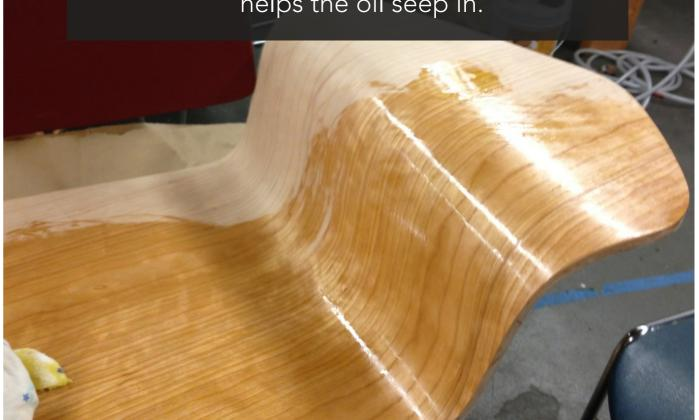
For aesthetics I added a top and a bottom layer of Cherry veneers. I had done 8 layers in my main middle section, but it was still pretty flexible. Adding these two layers vastly increased its strength, especially since the grain ran in a different direction.
