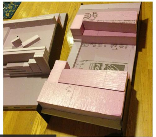
→ If you are using the wire cutter, **DO NOT USE PINK FOAM**. It is way stiffer than the white foam, which would seem like a good idea, but actually just breaks the wire very quickly. I went through over 20 wires to cut the buck, which made the process take over 6 hours.
